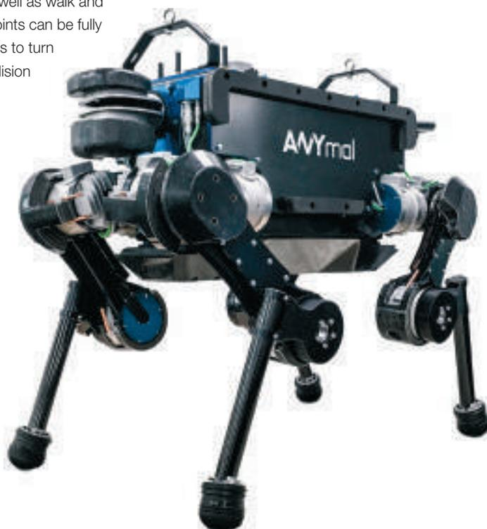
protection housing, foam absorbs the impact of side falls and a Kevlar belly protects from sharp objects below. The main body holds the computers, batteries, network devices, power management system and navigational sensors. It is sealed against water and dust ingress, complying to IP-67 standards.
